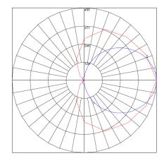
Luminaire Efficacy Rating (LER) 84 Maximum Candela 495.18 Maximum Candela Angle 0H 87.5V Cutoff Classification (deprecated) Non-Cutoff
