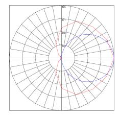
Luminaire Efficacy Rating (LER) 84 Maximum Candela 495.18 Maximum Candela Angle 0H 87.5V **Cutoff Classification** (deprecated) Non-Cutoff
