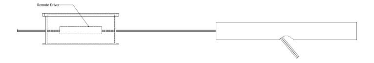
• Step 4: Connect the two wires of the light fixture to the cable inside the handrail in parallel circuit.
